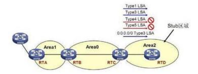
Set stub rear region, to produce a three lsa default route, the default route metric similar import external routes RTD interface cost is set to 2, the effect in question can reach
