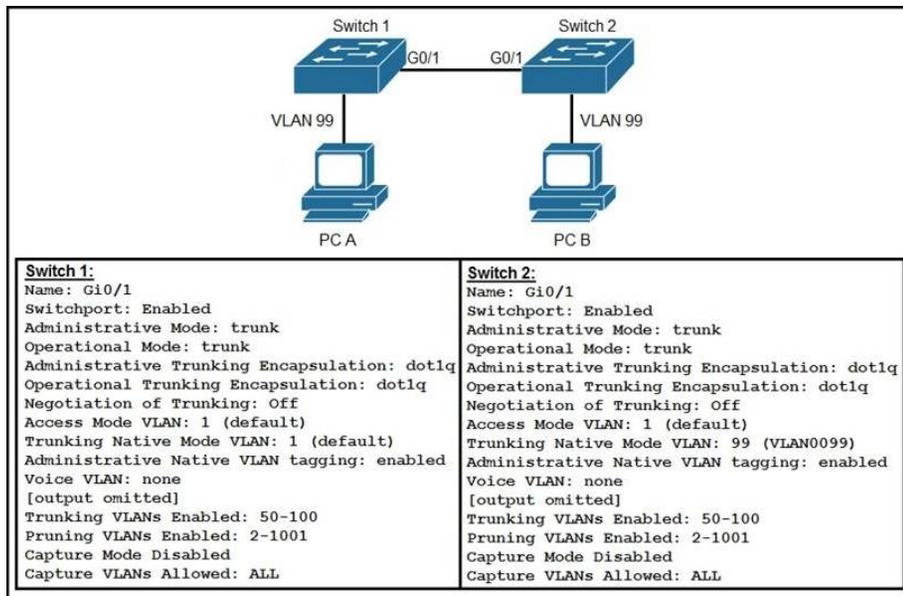
After the switch configuration, the ping test fails between PC A and PC B.
