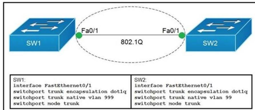
Which action do the switches take on the trunk link?
